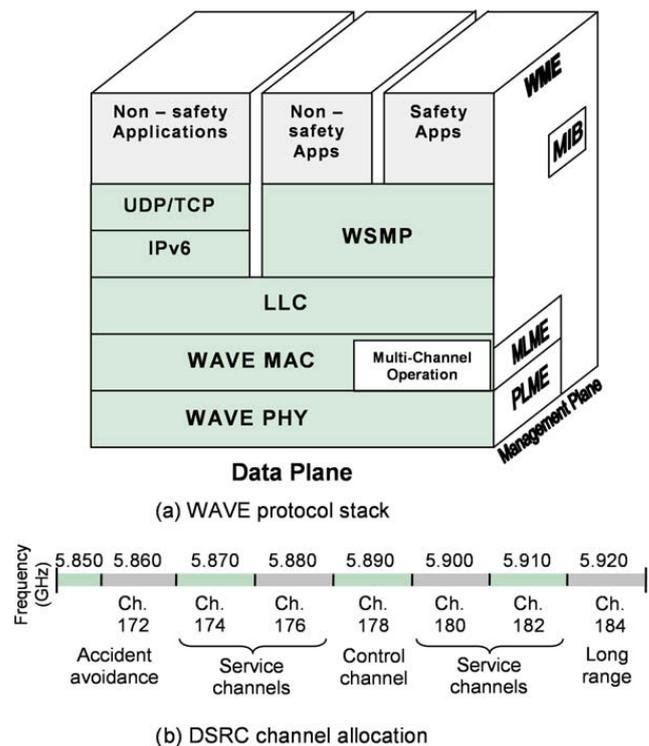
Fig. 1. WAVE protocol stack and DSRC channel allocation.
